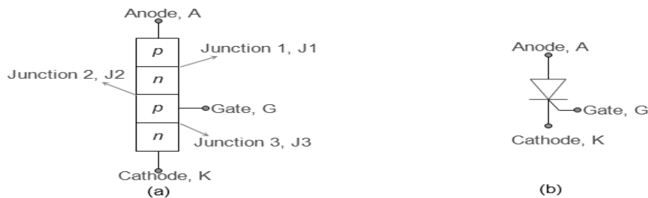
Figure 1 Silicon Controlled Rectifier (a) Layered Structure (b) Symbol
